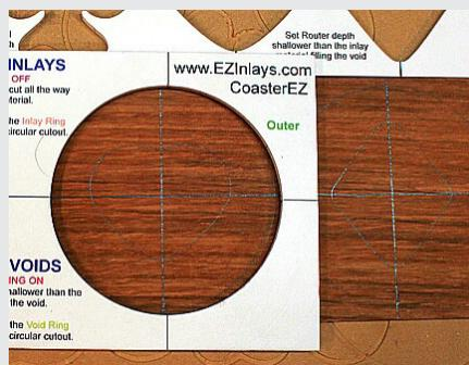
**2** Align & tape each card shape to Base Material. Cut voids using Cutting Voids procedure.
