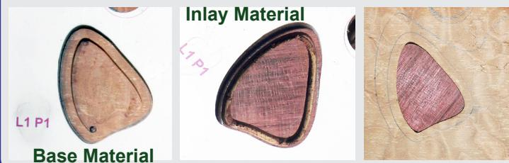
**4** Align & tape Layer 3 to Base Material. Cut voids using Cutting Voids procedure. Align & tape L3P1, L3P2, L3P3, and L3P4 to Inlay Materials. Cut inlays using Cutting Inlays procedure. Assemble inlays into voids.
