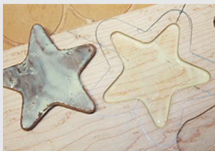
**8 Align & tape Pattern 3 to Base Material. Cut inlay using Cutting Inlays procedure.**
