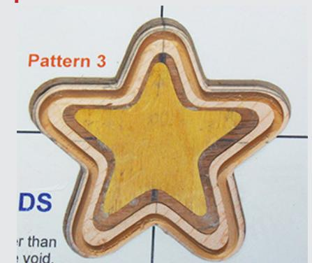
**9 Fill gaps with glue and sand. Sand to desired smoothness and apply finish.**
